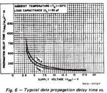
g. 6 -- Typical data propagation delay time vs. supply voltage.
