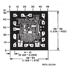
Dimensions in parentheses are in millimeters and are derived from the basic inch dimensions as indicated. Grid graduations are in mils (10<sup>-3</sup> inch).
