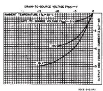
Fig. 5 – Minimum output high (source) current characteristics. 3
