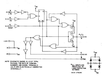
Fig. 4 - CD4098B logic diagram.
