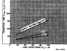
Fig. 7 – Transition time vs. load capacitance for  $R_X = 5 k\Omega \cdot 10000 k\Omega$  and  $C_X = 15 pF \cdot 10000 pF$ .
