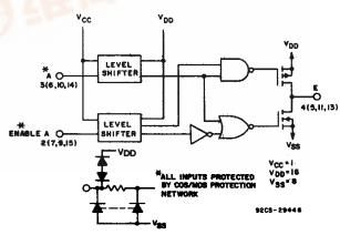
Fig.1 - CD40109B logic diagram (1 of 4 units).
