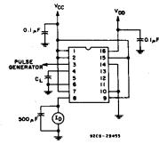
Fig. 16 - Dynamic power dissipation test circuit.
