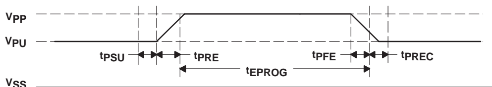
Figure 16. Program Pulse Timing Diagram
