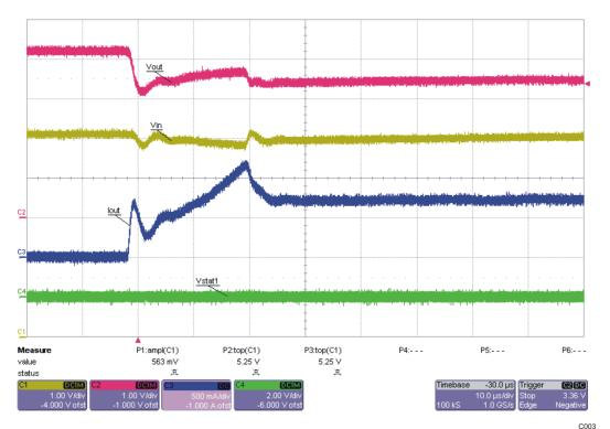
Figure 4. Battery Hot-Plug During Charging Phase
