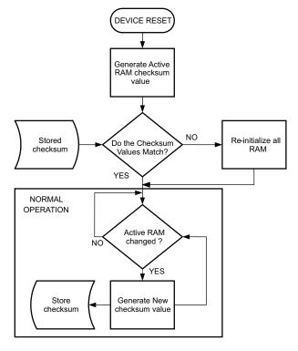
Figure 5-2. Partial Reset Flow Diagram
