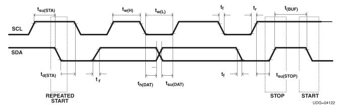
Figure 3-1. I<sup>2</sup>C-Compatible Interface Timing Diagrams
