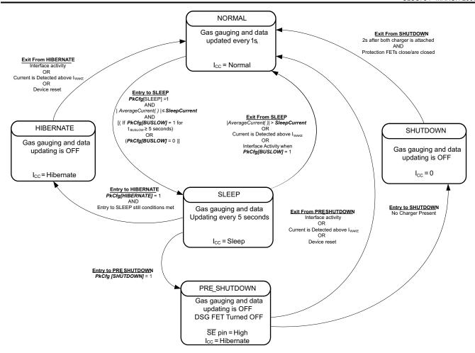
Figure 5-1. Power Mode Diagram
