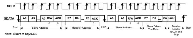
Figure 6. I<sup>2</sup>C-Bus Read from bg29330: Protocol A
