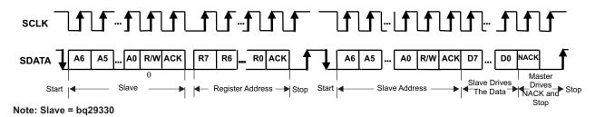
Figure 7. I<sup>2</sup>C-Bus Read from bq29330: Protocol B
