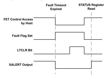
Figure 1. LTCLR and XLAERT Clear Timing
