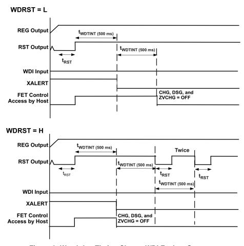
Figure 3. Watchdog Timing Chart - WDI Fault at Start-up
