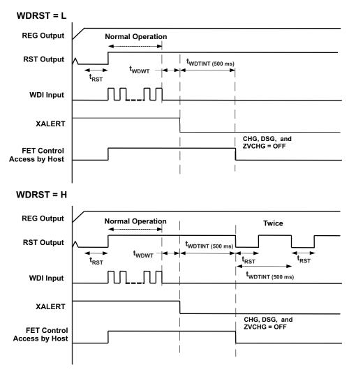
Figure 4. Watchdog Timing Chart – WDI Fault After Startup
