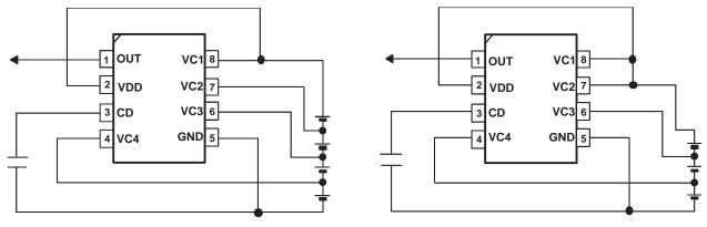
Figure 3. 4-Series Cell Configuration
