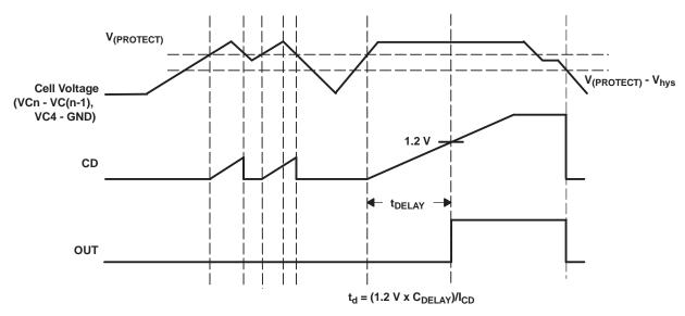
Figure 2. Timing for Overvoltage Sensing
