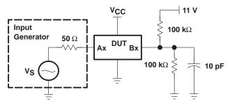
Figure 1. Device Test Setup
