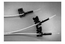
To install *simplex* connectors flip the top half of the connector over and snap it into the ferrule half (with your fingers). When the top half latches inside the body of the ferrule half, proper connector-to-cable attachment is achieved.
