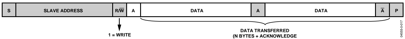
Figure 17. I 2 C—Master Reading Data from Slave
