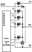
Figure 4. AD5280/AD5282 Equivalent RDAC Circuit
