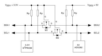
Figure 6. Level Shift for different potential operation.
