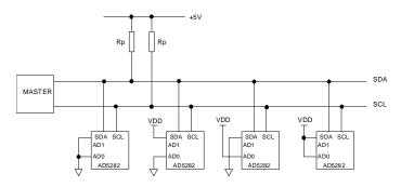
Figure 5. Multiple AD5282 Devices on One Bus
