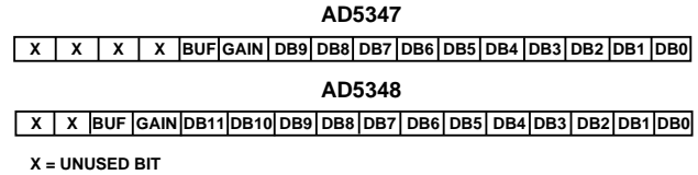
Figure 40. AD5347/AD5348 Data Format for Word Load with GAIN and BUF Data on 16-Bit Bus
