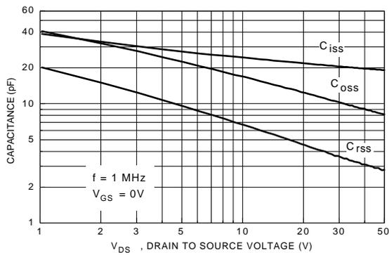
Figure 9. Capacitance Characteristics.
