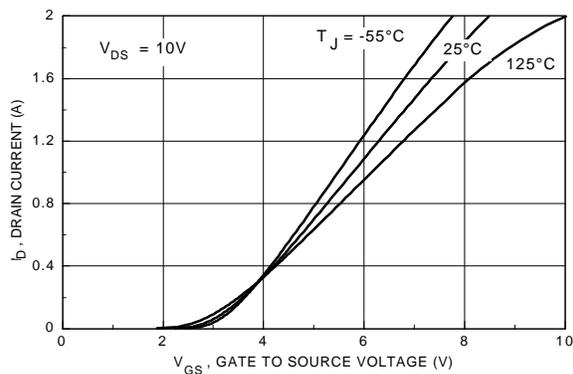
Figure 5. Transfer Characteristics.
