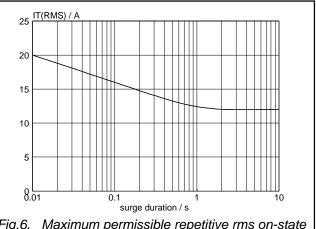
Fig.6. Maximum permissible repetitive rms on-state current  $I_{T(RMS)}$ , versus surge duration, for sinusoidal currents, f = 50 Hz;  $T_{mb} \le 103$  °C.
