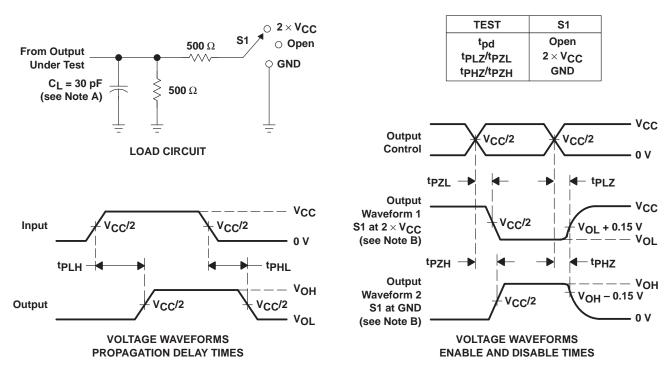
NOTES: A. C<sub>I</sub> includes probe and jig capacitance.
