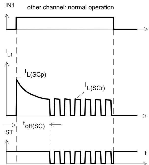
Heating up of the chip may require several milliseconds, depending on external conditions ( $t_{off(SC)}$  vs.  $T_{j,start}$  see page 10)
