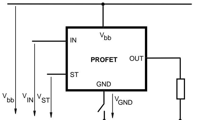
In case of  $IN=high$  is  $V_{OUT} \approx V_{IN} - V_{IN(T+)}$ . Due to  $V_{GND} > 0$ , no  $V_{ST} = \text{low}$  signal available.
