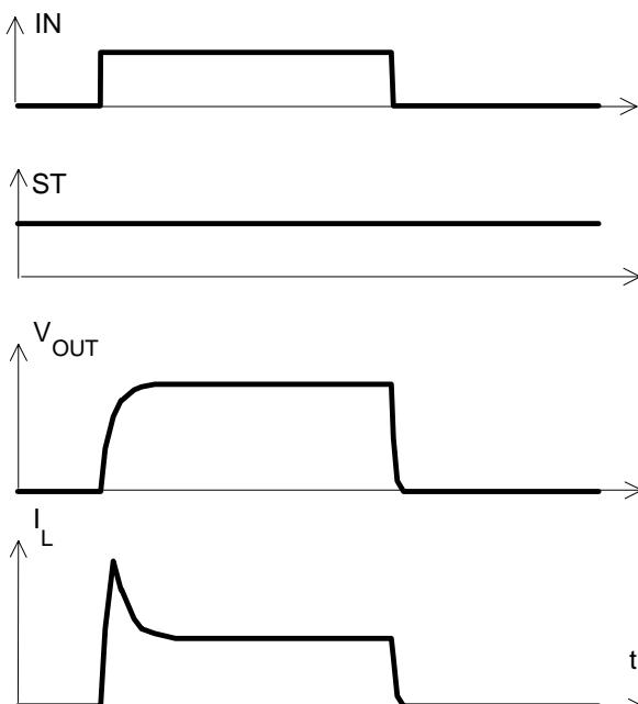
The initial peak current should be limited by the lamp and not by the initial short circuit current  $I_{L(SCp)} = 28$  A typ. of the device.
