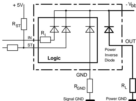
$R_{GND} = 150 \Omega$ ,  $R_I = 3.5 \text{ k}\Omega$  typ,
