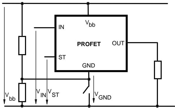
If  $V_{GND} > V_{IN} - V_{IN(T+)}$  device stays off
