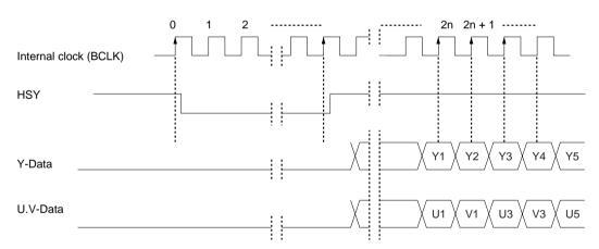
Fig. 25 YUV input timing when TEST[2] = L
