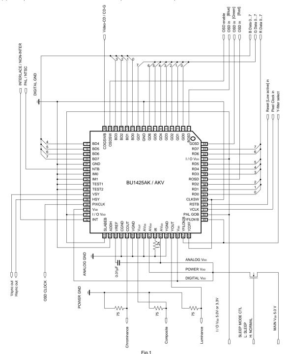
(2) Example in Slave mode: Doubled clock is input and 16-bit YUV input is used
