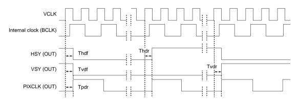
Fig. 16 Output timing with a doubled clock
