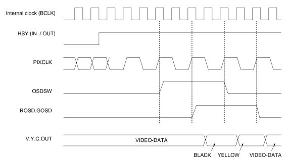
Fig. 15 Clock timing with the OSD function
