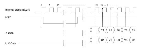
Fig. 26 YUV input timing when TEST[2] = H
