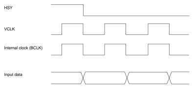
Fig. 4 Illustration of clock timing (CLKSW is HIGH)
