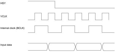
Also, setting the CLKSW pin to HIGH enables the frequency of the external clock to be used as BCLK, the internal clock, just as it is. Since the data is read to the
