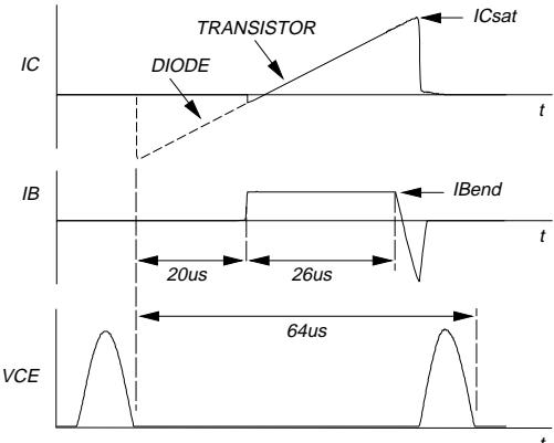
Fig.1. Switching times waveforms.
