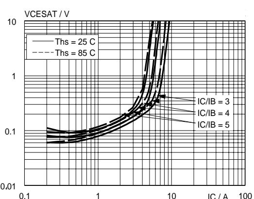
Fig.6. Typical collector-emitter saturation voltage.
