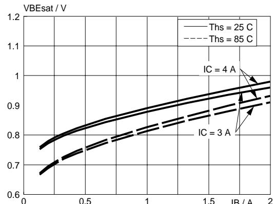
Fig.7. Typical base-emitter saturation voltage.
