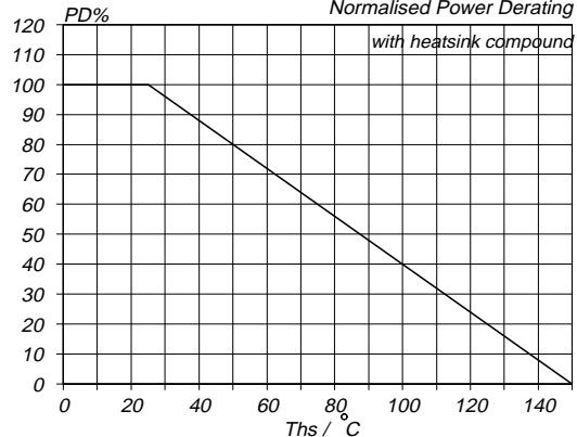
Fig.10. Normalised power dissipation.
