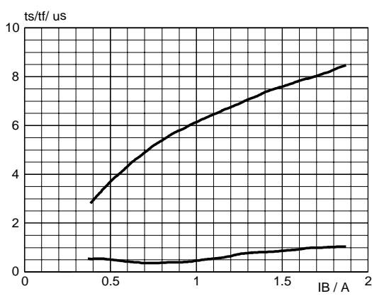
Fig.9. Typical collector storage and fall time.
