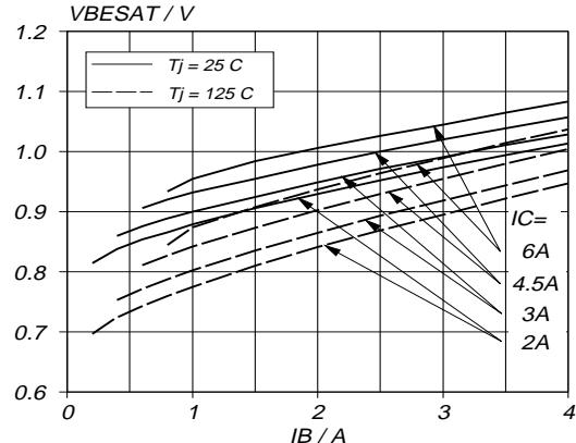
Fig.7. Typical base-emitter saturation voltage.
