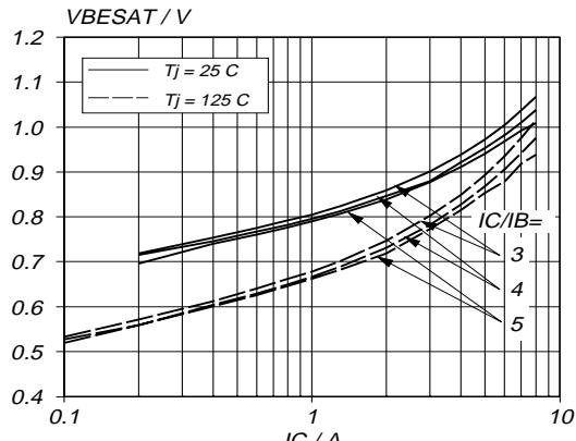
Fig.5. Typical base-emitter saturation voltage.  $V_{BE\text{sat}} = f (I_C)$ ; parameter  $I_C/I_B$
