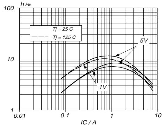
Fig.4. Typical DC current gain.  $h_{FE} = f (I_C)$  parameter  $V_{CE}$
