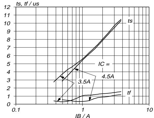
Fig.10. Typical collector storage and fall time.
