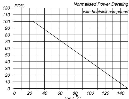
Fig.11. Normalised power dissipation.
