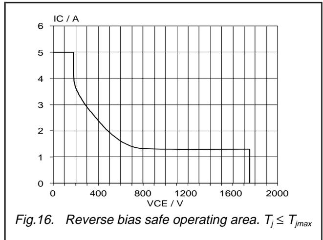
Fig.16. Reverse bias safe operating area.  $T_j \leq T_{jmax}$
