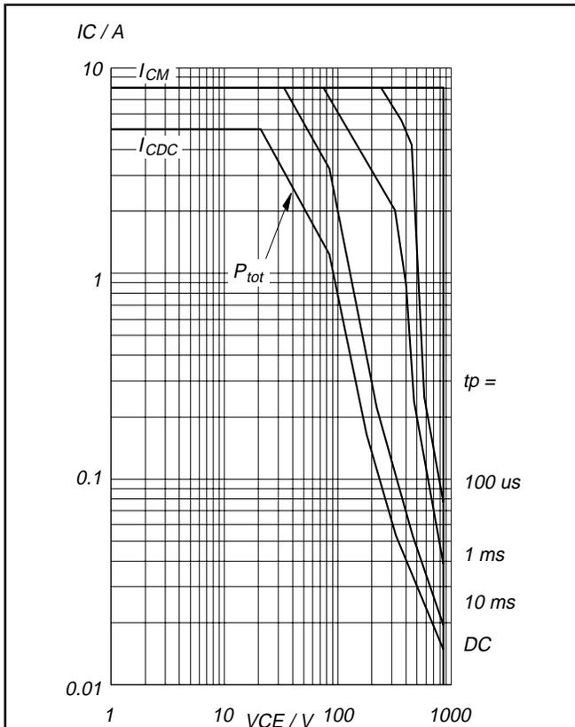
Fig.15. Forward bias safe operating area.  $T_{mb} = 25^\circ\text{C}$
