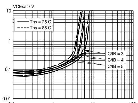
Fig.6. Typical collector-emitter saturation voltage.
