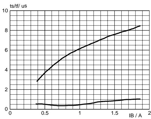
Fig.9. Typical collector storage and fall time.
