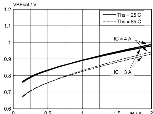
Fig.7. Typical base-emitter saturation voltage.
