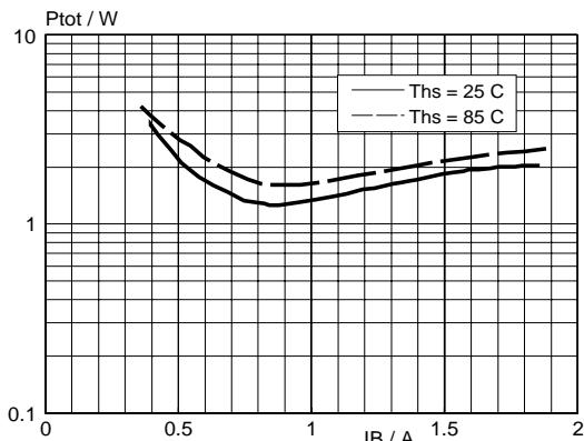
Fig.8. Typical losses.
