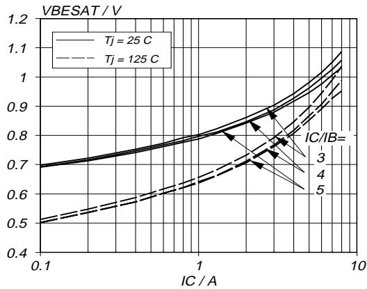
Fig.7. Typical base-emitter saturation voltage.
