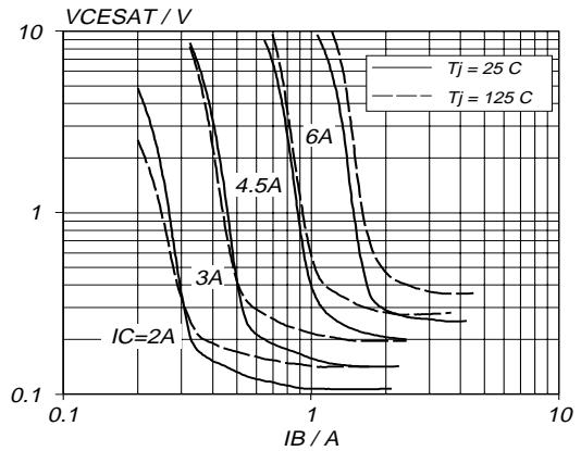
Fig.10. Typical collector-emitter saturation voltage.
