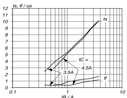
Fig.12. Typical collector storage and fall time.
