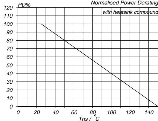
Fig. 13. Normalised power dissipation.
