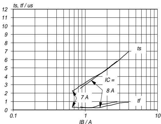
Fig.12. Typical collector storage and fall time.
