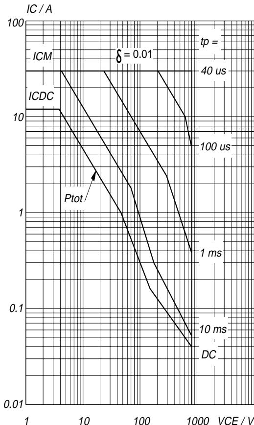
Fig. 15. Forward bias safe operating area.  $T_{hs} = 25^\circ C$
