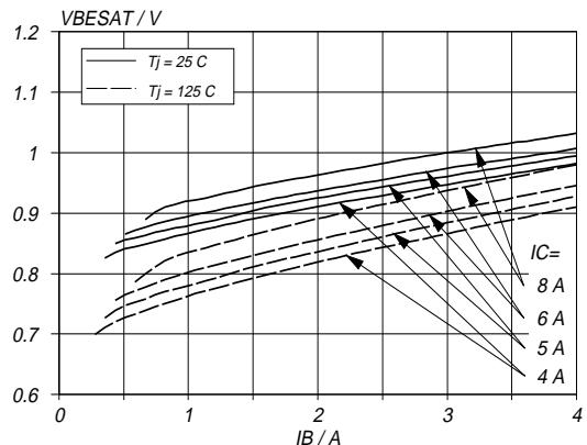
Fig.9. Typical base-emitter saturation voltage.
