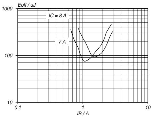
Fig.11. Typical turn-off losses.  $T_j = 85^\circ C$
