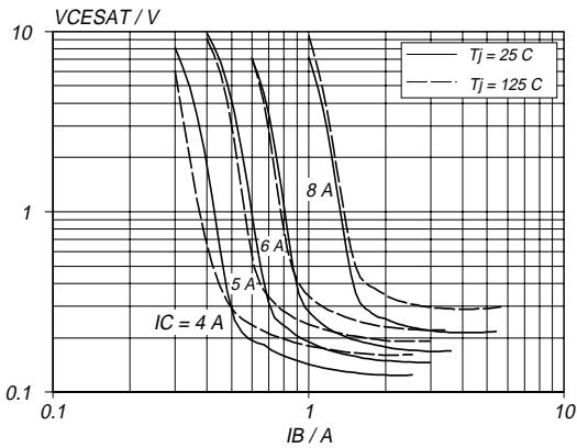
Fig.10. Typical collector-emitter saturation voltage.
