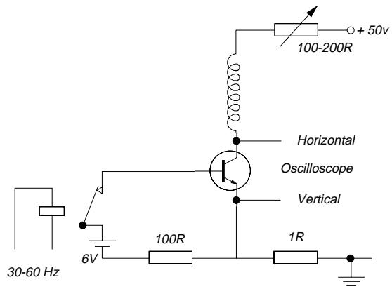
Fig.1. Test circuit for  $V_{CEO}^{sust}$ .
