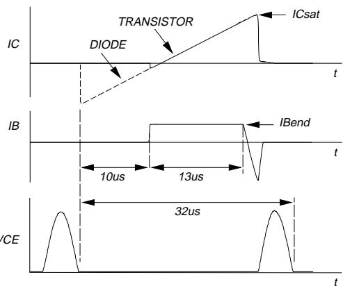
Fig.3. Switching times waveforms.
