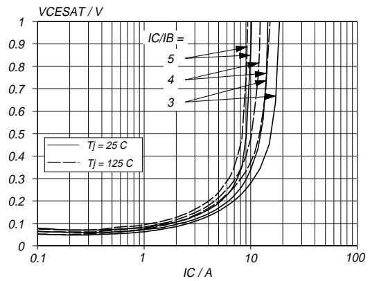
Fig.8. Typical collector-emitter saturation voltage.
