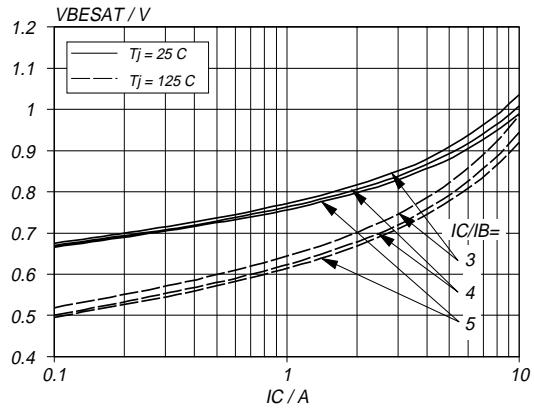
Fig.7. Typical base-emitter saturation voltage.
