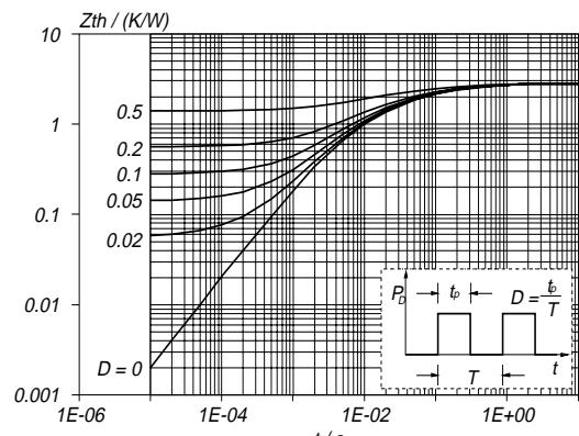
Fig. 14. Transient thermal impedance.
