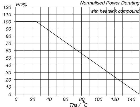
Fig.13. Normalised power dissipation.
