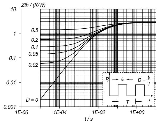
Fig.14. Transient thermal impedance.
