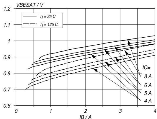
Fig.9. Typical base-emitter saturation voltage.
