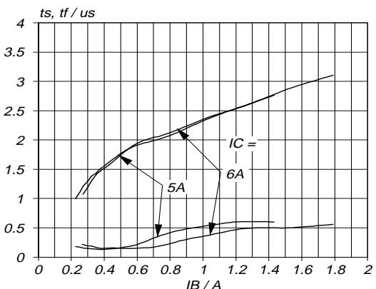
Fig.12. Typical collector storage and fall time.
