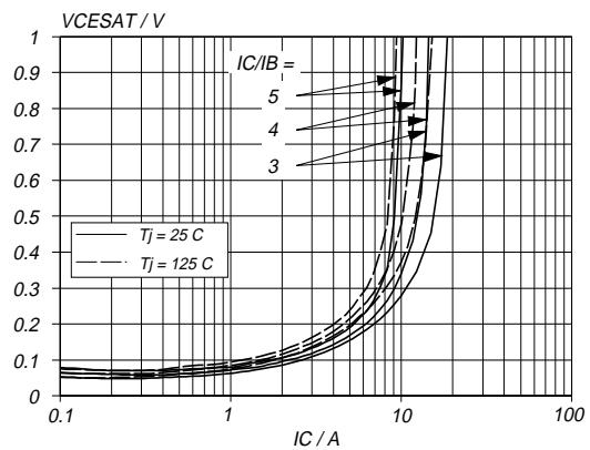
Fig.8. Typical collector-emitter saturation voltage.
