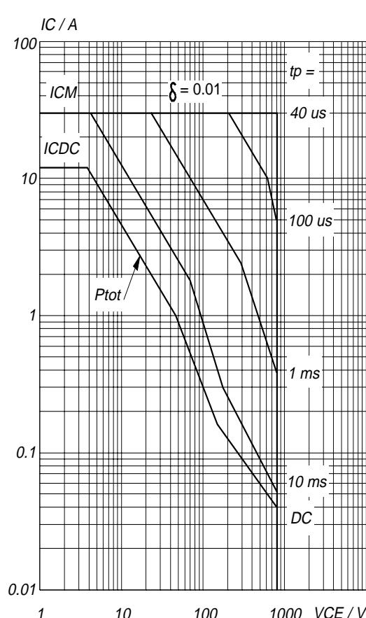
Fig.16. Forward bias safe operating area.  $T_{hs} = 25^\circ C$
