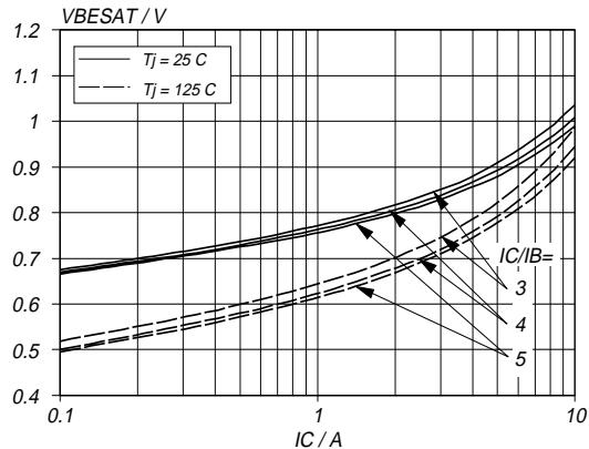
Fig.7. Typical base-emitter saturation voltage.
