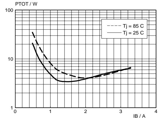
Fig.8. Typical turn-off losses.
