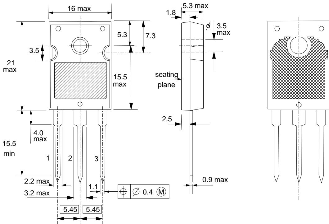
Fig.14. SOT429; pin 2 connected to mounting base.
