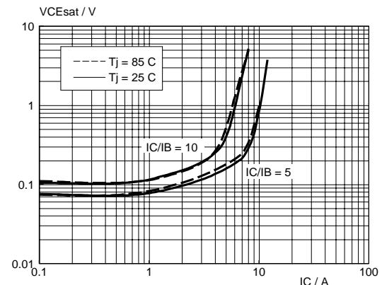
Fig.6. Typical collector-emitter saturation voltage.
