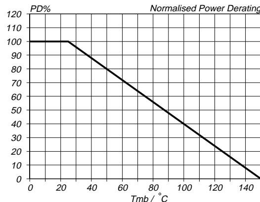
Fig.10. Normalised power dissipation.
