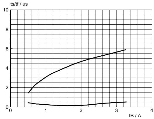
Fig.9. Typical collector storage and fall time.
