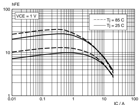
Fig.4. High and low DC current gain.  $h_{FE} = f(I_C)$
