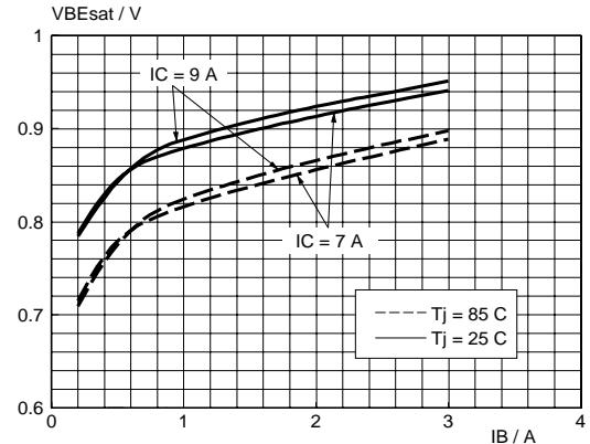
Fig.7. Typical base-emitter saturation voltage.
