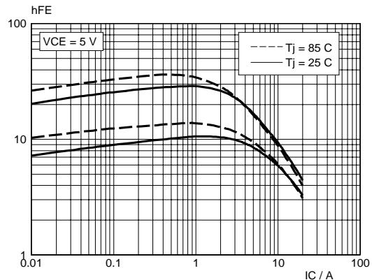
Fig.5. High and low DC current gain.  $h_{FE} = f(I_C)$
