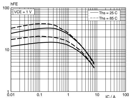
Fig.7. DC current gain.  $h_{FE} = f(I_C)$
