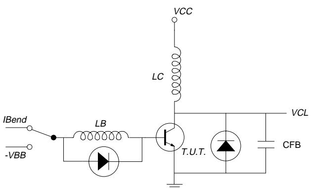
Fig.14. Test Circuit RBSOA.  $V_{CC} = 150 \text{ V}$ ;
