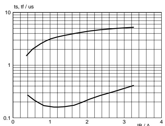
Fig.12. Typical storage and fall time.
