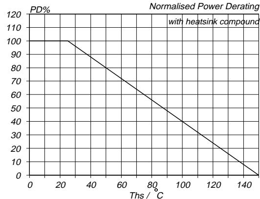
Fig.10. Normalised power dissipation.
