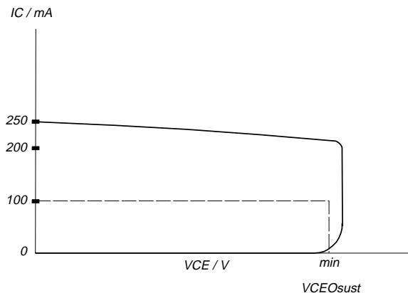
Fig.2. Oscilloscope display for  $V_{CEO}sust$ .
