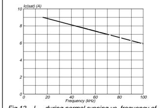
Fig.12. I<sub>Csat</sub> during normal running vs. frequency of operation for optimum performance
