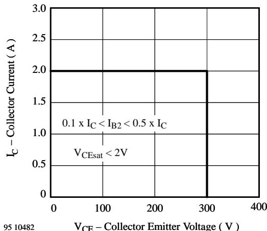
Figure 4.  $V_{CEW}$  – Diagram
