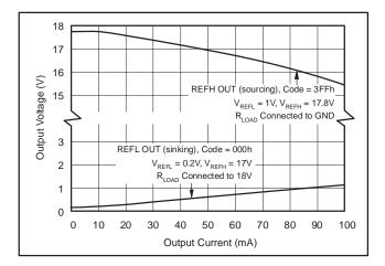
Figure 13. Reference Buffer Output Voltage vs Output Current
