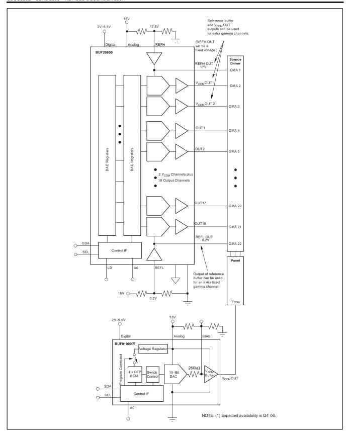
Figure 15. 22-Channel Gamma Solution
