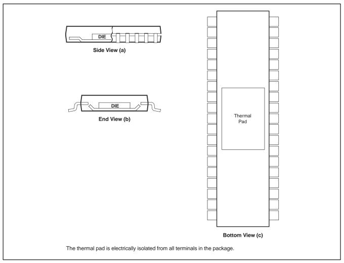
Figure 20. Views of Thermally-Enhanced DCP Package
