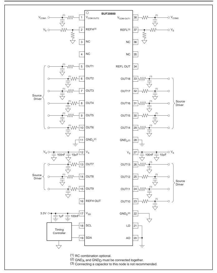
Figure 8. Typical Application Configuration
