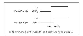
Figure 7. Power Supply Timing Requirements
