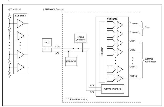
Figure 11. Replacement of the Traditional Gamma Buffer
