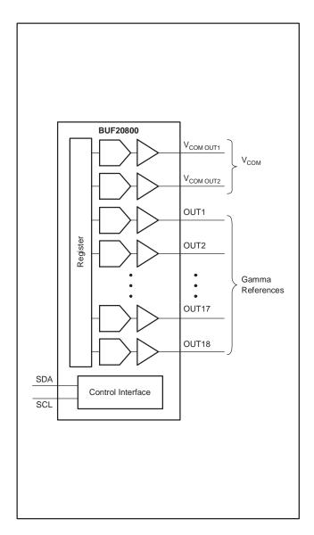
Figure 12. BUF20800 Used for Programmable  $V_{\text{COM}}$
