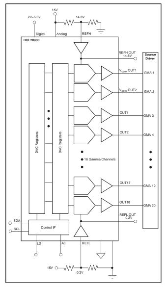
Figure 14. 20 Gamma Channel Solution – Two V<sub>COM</sub> Channels Used as Additional Gamma Channels
