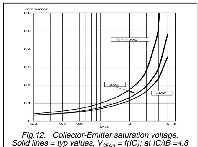
Silicon Diffused Power Transistor
