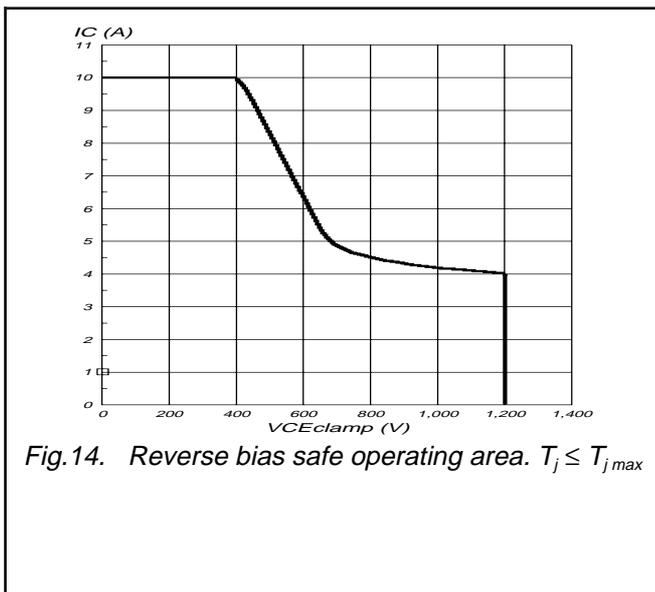
Silicon Diffused Power Transistor
