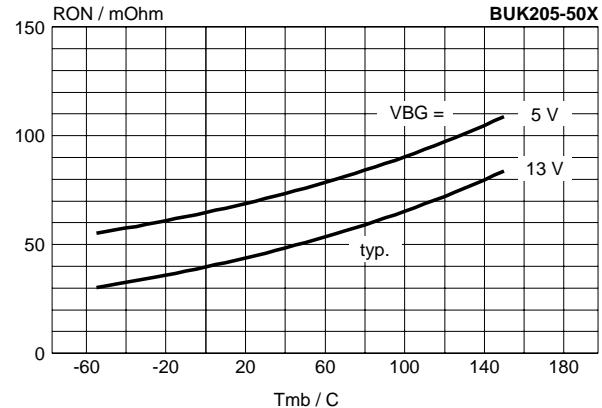
Fig.9. Typical on-state resistance,  $t_p = 300\ \mu\text{s}$ .
