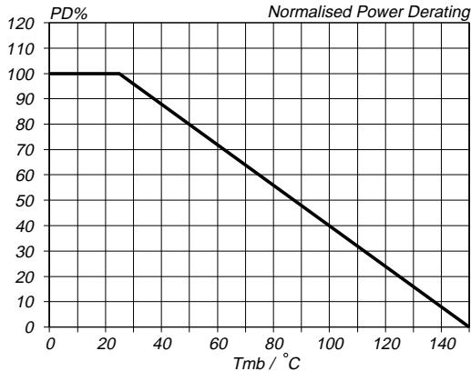
Fig.5. Normalised limiting power dissipation.
