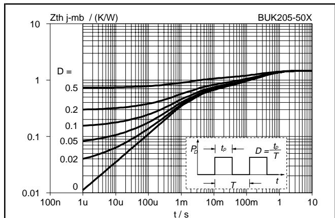
Fig.37. Transient thermal impedance.
