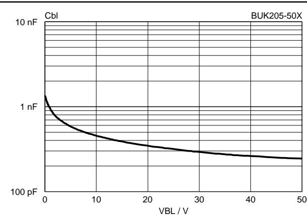
Fig.32. Typical output capacitance.  $T_{mb} = 25 ^\circ C$
