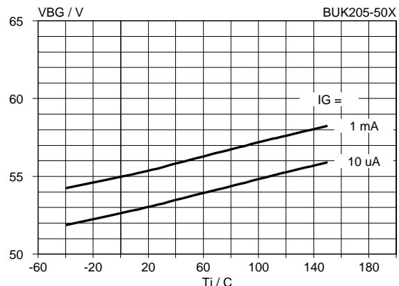
Fig.26. Typical battery to ground clamping voltage.
