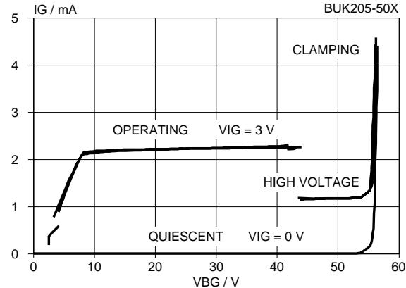
Fig.10. Typical supply characteristics, 25 °C.
