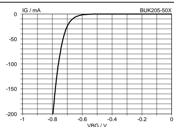
Fig.30. Typical reverse battery characteristic.
