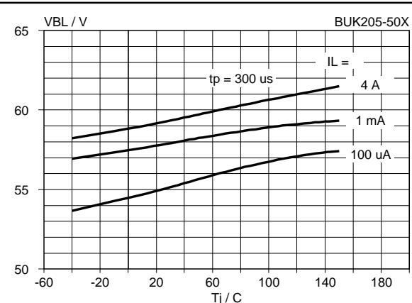
Fig.29. Typical battery to load clamping voltage.
