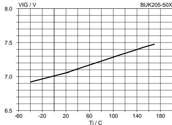
Fig.17. Typical input clamping voltage.
