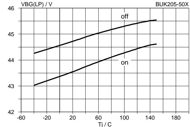
Fig.25. Supply typical overvoltage thresholds.
