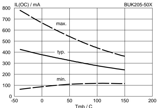
Fig.23. Low load current detection threshold.
