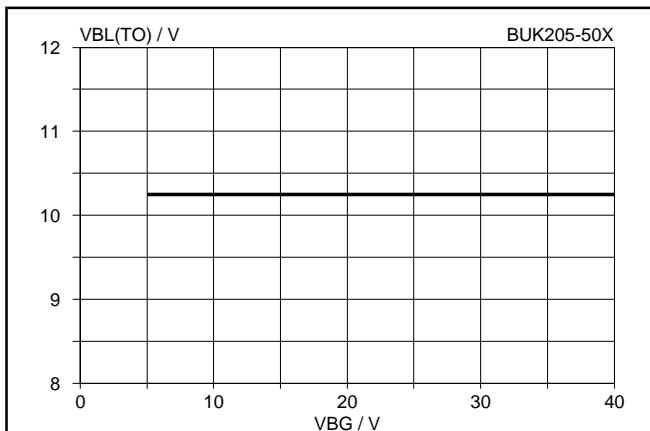
Fig.35. Typical short circuit load threshold voltage.
