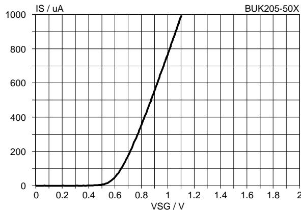
Fig.20. Typical status low characteristic,  $T_j = 25^\circ\text{C}$ .
