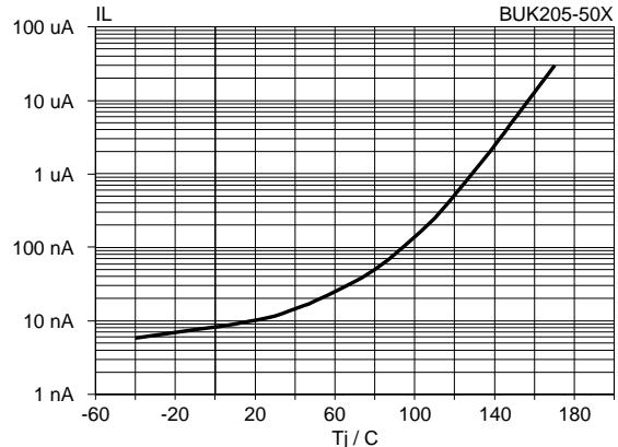
Fig.13. Typical off-state leakage current.
