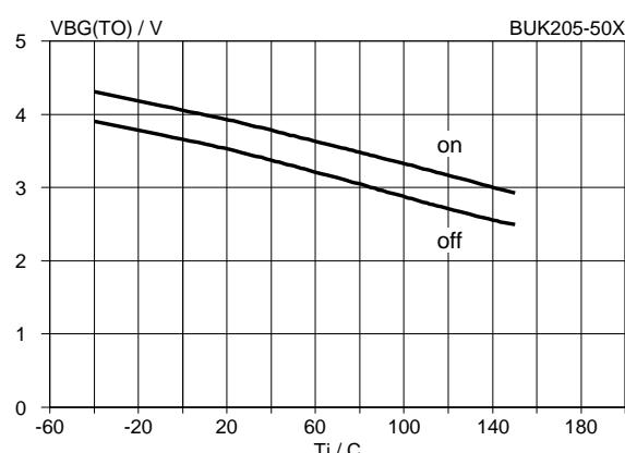
Fig.24. Supply typical undervoltage thresholds.
