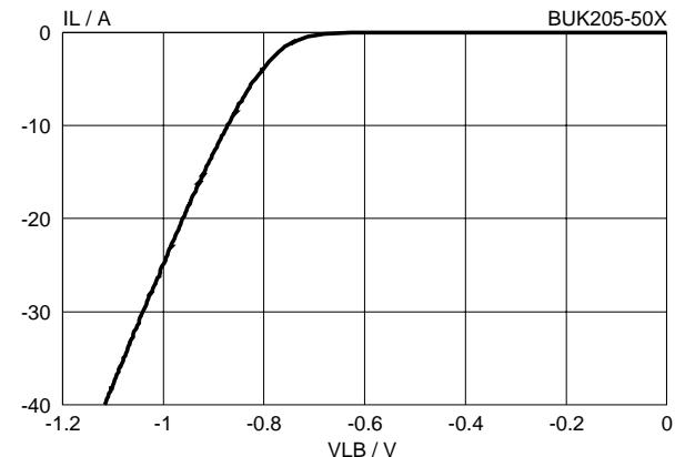
Fig.31. Typical reverse diode characteristic.
