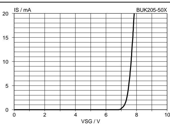
Fig.18. Typical status characteristic,  $T_j = 25^\circ\text{C}$ .
