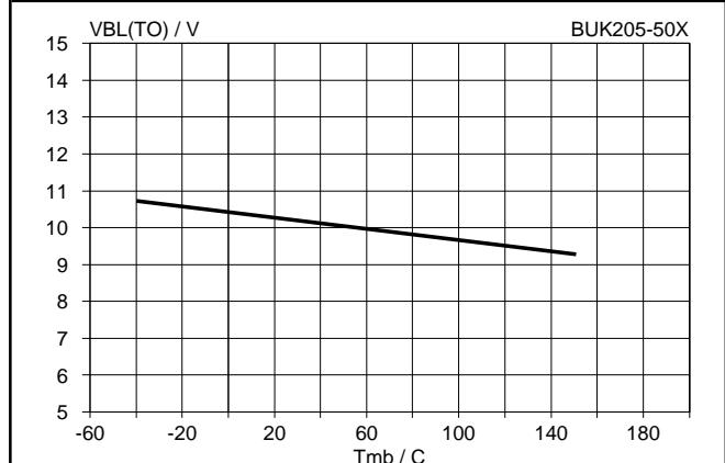
Fig.36. Typical short circuit load threshold voltage.
