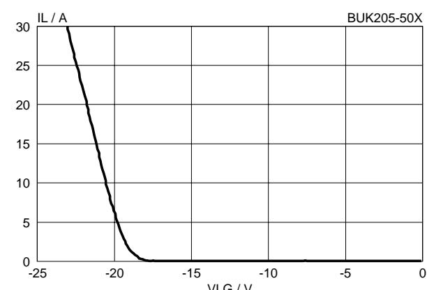
Fig.27. Typical negative load clamping characteristic.
