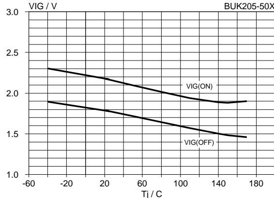
Fig.16. Typical input threshold voltages.
