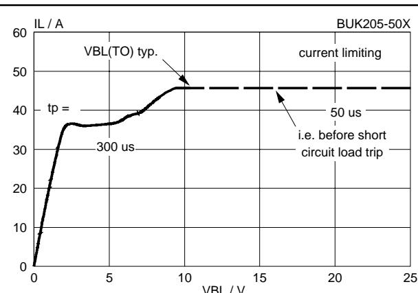
Fig.33. Typical overload characteristic,  $T_{mb} = 25 ^\circ C$ .
