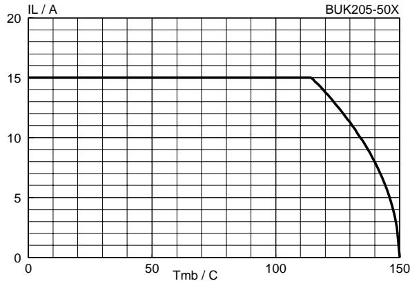
Fig.6. Limiting continuous on-state load current.
