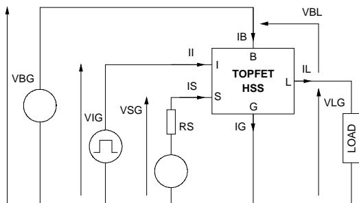
Fig.4. High side switch measurements schematic.
