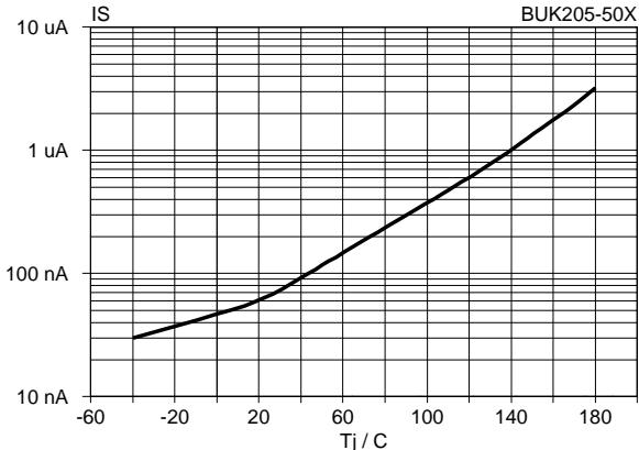
Fig.19. Typical status leakage current.
