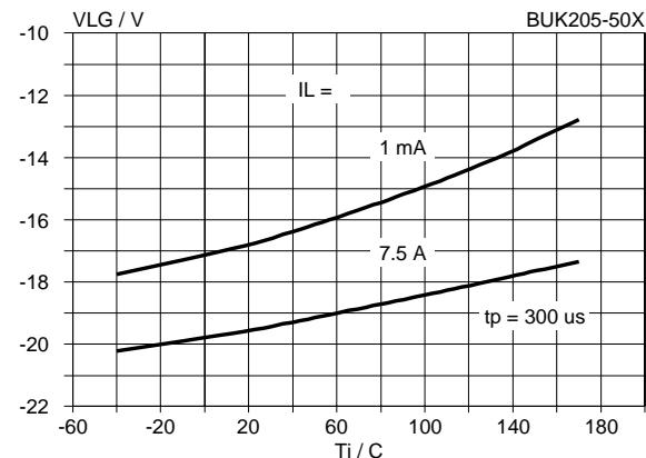
Fig.28. Typical negative load clamping voltage.
