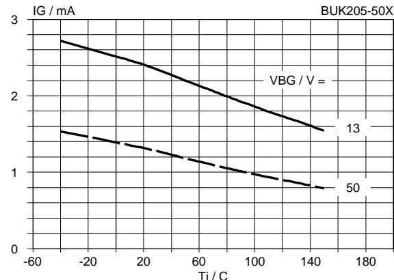
Fig.11. Typical operating supply current.
