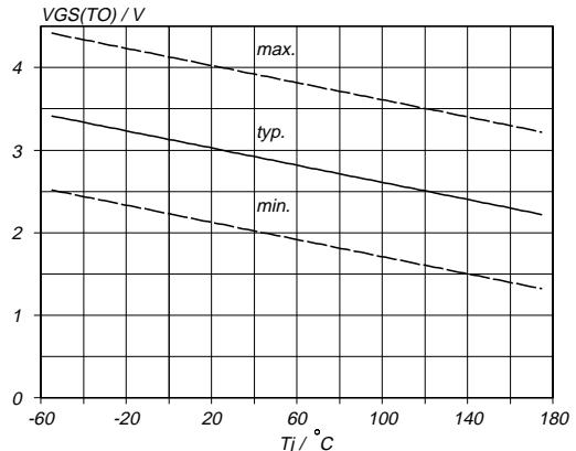
Fig.10. Gate threshold voltage.
