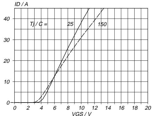
Fig.7. Typical transfer characteristics.
