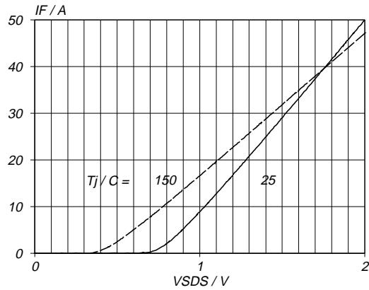
Fig.14. Typical reverse diode current.
