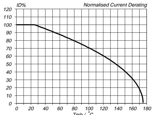
Fig.2. Normalised continuous drain current.
