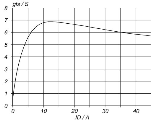
Fig.8. Typical transconductance,  $T_j = 25^\circ\text{C}$ .
