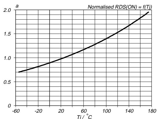
Fig.9. Normalised drain-source on-state resistance.
