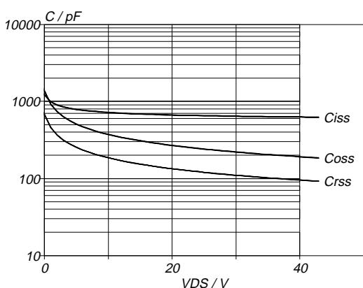
Fig.12. Typical capacitances,  $C_{iss}$ ,  $C_{oss}$ ,  $C_{rss}$ .
