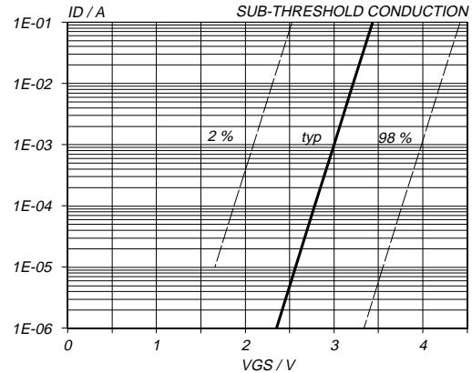
Fig.11. Sub-threshold drain current.
