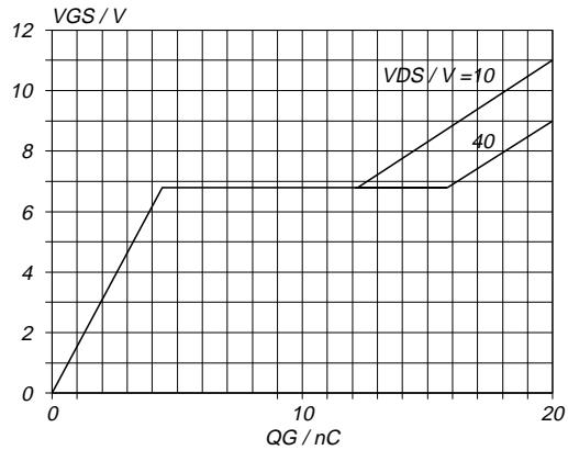
Fig.13. Typical turn-on gate-charge characteristics.
