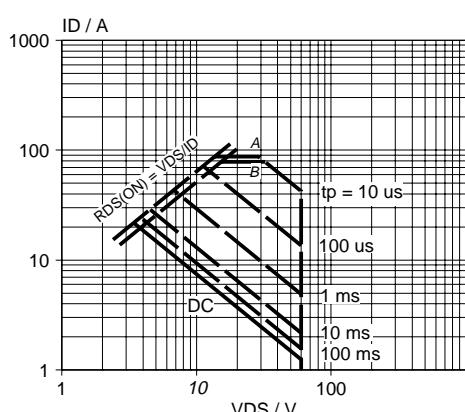
Fig.3. Safe operating area.  $T_{mb} = 25\ ^{\circ}\text{C}$
