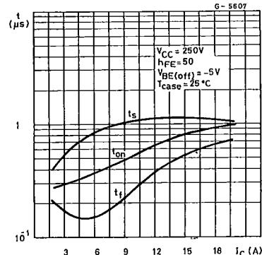
Switching Times Inductive Load Test (test circuit fig. 1).
