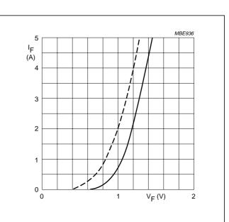
Dotted line:  $T_j = 150 \text{ °C}$ ; solid line:  $T_j = 25 \text{ °C}$ .
