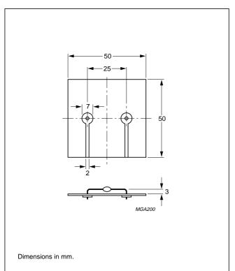
Fig.4 Device mounted on a printed-circuit board.
