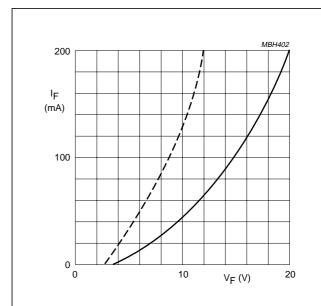
Dotted line:  $T_j = 120 \,^{\circ}\text{C}$ . Solid line:  $T_j = 25 \,^{\circ}\text{C}$ .
