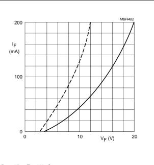
Dotted line:  $T_j = 120 \ ^{\circ}C$ . Solid line:  $T_j = 25 \ ^{\circ}C$ .
