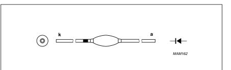
The cathode lead is marked with an orange band.
