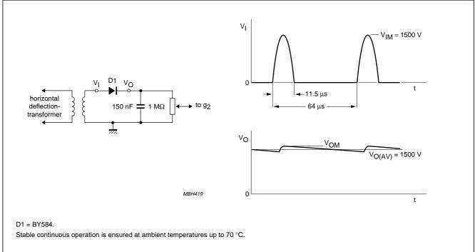
Fig.8 Basic circuit and waveforms for grid 2 voltage supply in colour television picture tubes.
