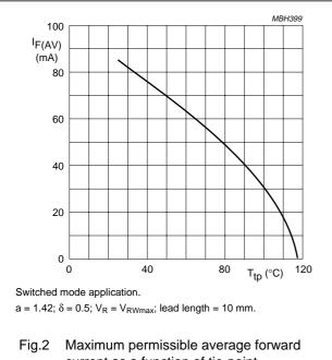
Fig.2 Maximum permissible average forward current as a function of tie-point temperature (including losses due to reverse leakage).
