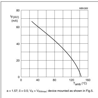
Fig.2 Maximum permissible average forward current as a function of ambient temperature (including losses due to reverse leakage).
