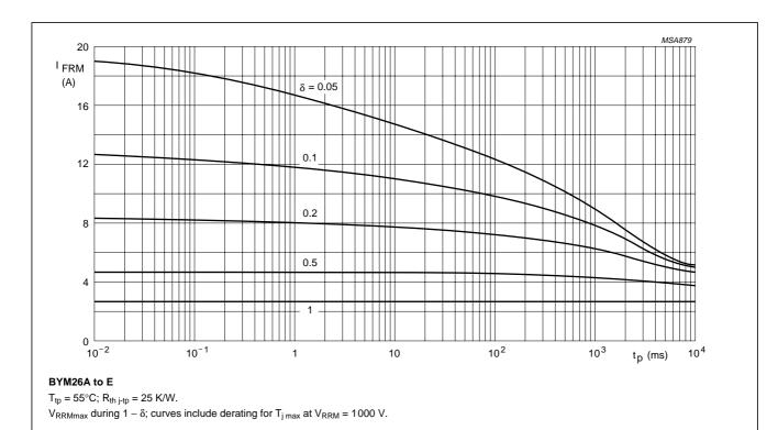
Fig.6 Maximum repetitive peak forward current as a function of pulse time (square pulse) and duty factor.
