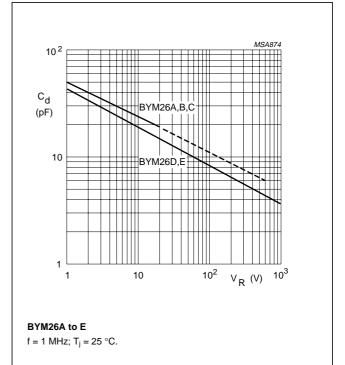
Fig.17 Diode capacitance as a function of reverse voltage; typical values.
