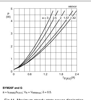
Fig.11 Maximum steady state power dissipation (forward plus leakage current losses, excluding switching losses) as a function of average forward current.
