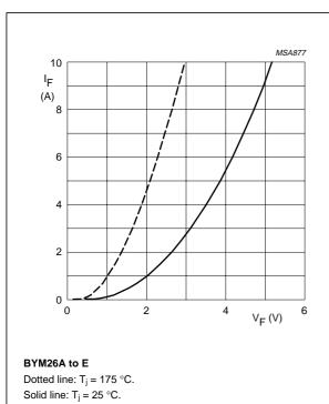
Fig.14 Forward current as a function of forward voltage; maximum values.
