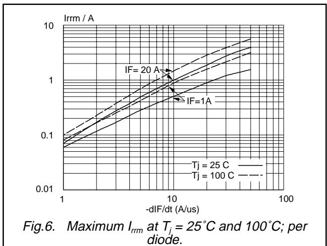
Fig.6. Maximum  $I_{rrm}$  at  $T_j = 25^\circ\text{C}$  and  $100^\circ\text{C}$ ; per diode.
