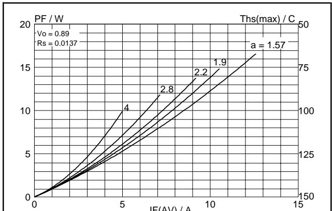
Fig.4. Maximum forward dissipation  $P_F = f(I_{F(AV)})$  per diode; sinusoidal current waveform where  $a = \text{form factor} = I_{F(\text{RMS})} / I_{F(\text{AV})}$ .
