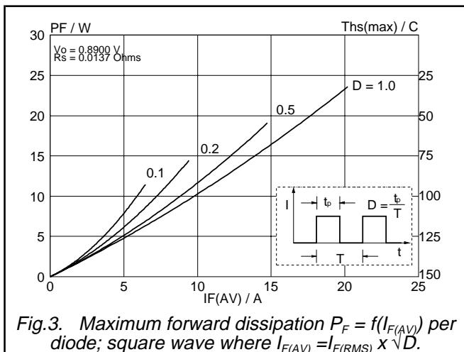
Fig.3. Maximum forward dissipation  $P_F = f(I_{F(AV)})$  per diode; square wave where  $I_{F(AV)} = I_{F(\text{RMS})} \times \sqrt{D}$ .
