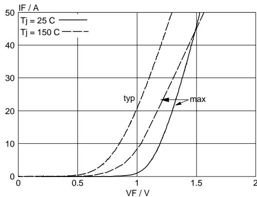
Fig.7. Typical and maximum forward characteristic
