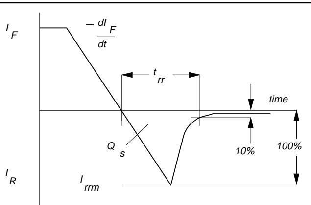
Fig.1. Definition of  $t_{rr}$ ,  $Q_s$  and  $I_{rrm}$
