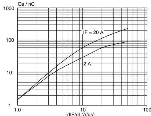
Fig.8. Maximum  $Q_s$  at  $T_j = 25^\circ\text{C}$ ; per diode
