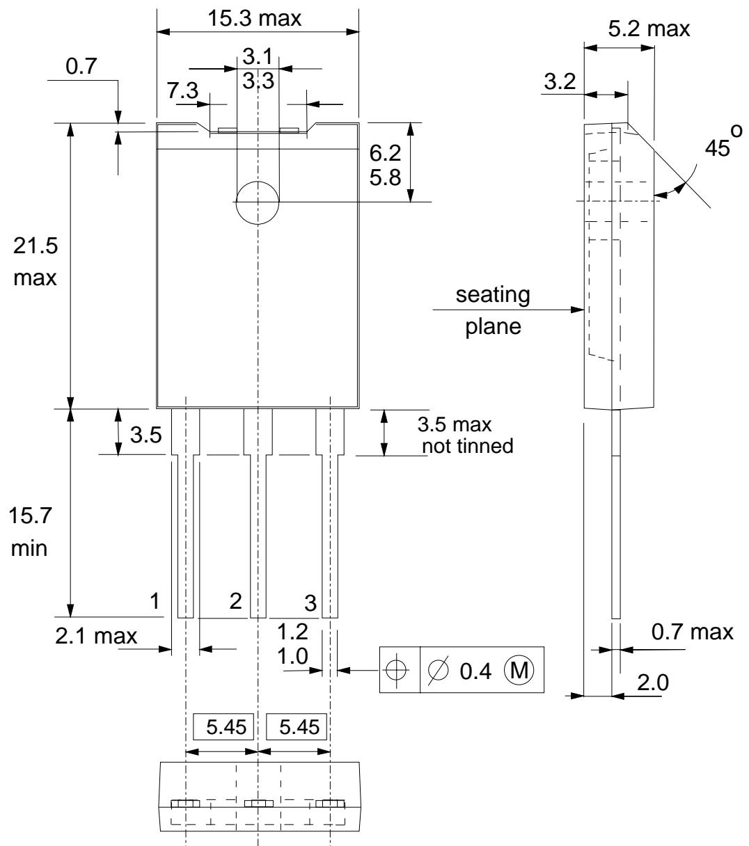
Fig.10. SOT199; The seating plane is electrically isolated from all terminals.
