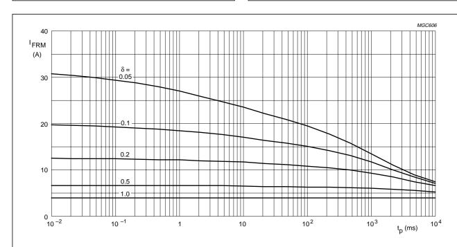
$T_{tp}$  = 60 °C;  $R_{th\ j-tp}$  = 25 K/W.
