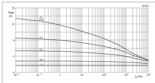
$$\begin{split} T_{amb} = 65 \text{ °C; } R_{th \text{ $j$-a}} = 75 \text{ K/W.} \\ V_{RRMmax} \text{ during } 1 - \delta; \text{ curves include derating for } T_{j \text{ max}} \text{ at } V_{RRM} = 600 \text{ V.} \end{split}$$
