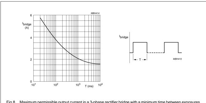
Fig.8 Maximum permissible output current in a 3-phase rectifier bridge with a minimum time between exposures of 20 s;  $T_{oil} = 50$  °C.
