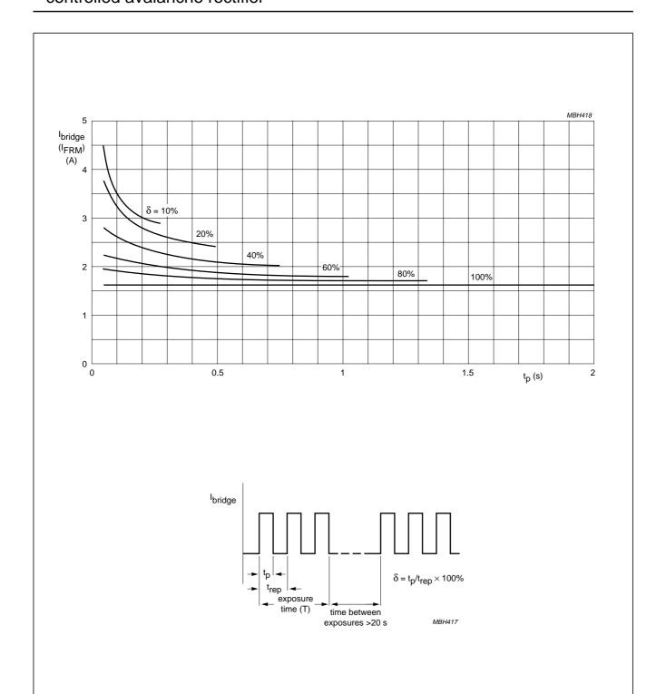
Fig.10 Maximum current through a 3-phase bridge rectifier versus pulse duration; exposure time T = 3 s;  $T_{oil}$  = 50 °C.
