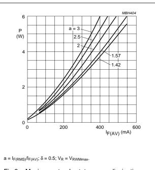
Fig.3 Maximum steady state power dissipation (forward plus leakage losses) as a function of average forward current.
