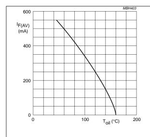
Fig.2 Maximum permissible average forward current as a function of oil temperature (including losses due to reverse leakage).
