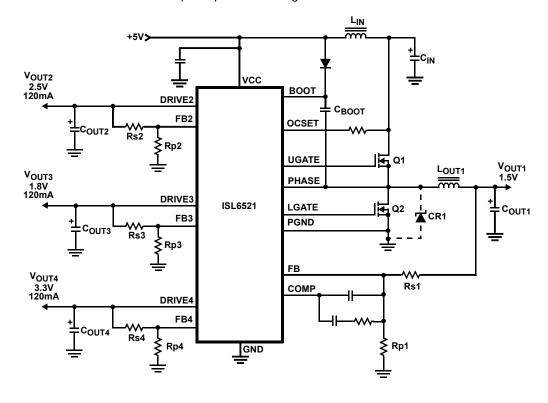
High Output Current PWM Converter and Auxiliary 3.3V Linear Regulator
