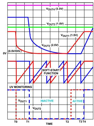
FIGURE 2. OVERCURRENT/UNDERVOLTAGE PROTECTION RESPONSE
