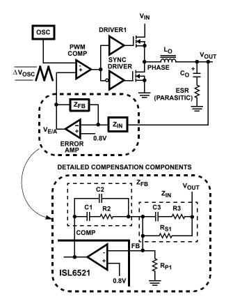
FIGURE 5. VOLTAGE-MODE BUCK CONVERTER COMPENSATION DESIGN
