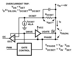
FIGURE 3. OVERCURRENT DETECTION
