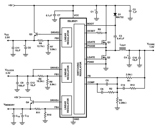
FIGURE 9. POWER SUPPLY APPLICATION CIRCUIT FOR AN EMBEDDED PROCESSOR
