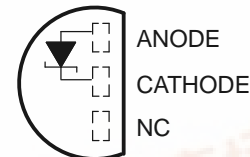
LP (TO-92/TO-226) PACKAGE (TOP VIEW)
