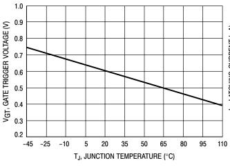
Figure 5. Typical Gate Trigger Voltage versus **Junction Temperature**
