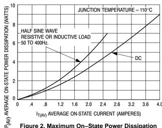
Figure 2. Maximum On-State Power Dissipation
