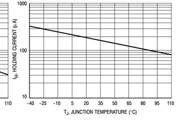
Figure 4. Typical Holding Current versus **Junction Temperature**
