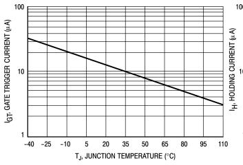
Figure 3. Typical Gate Trigger Current versus **Junction Temperature**
