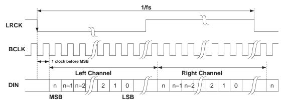
Figure 20. Timing Diagram for I2S Mode
