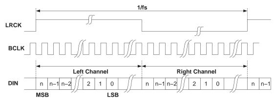
Figure 19. Timing Diagram for Left-Justified Mode
