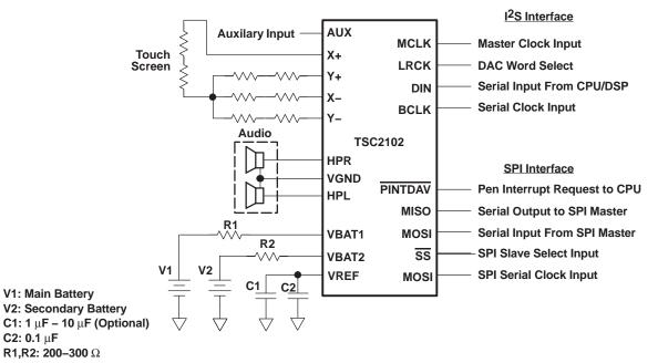
Figure 9. Typical Circuit Configuration
