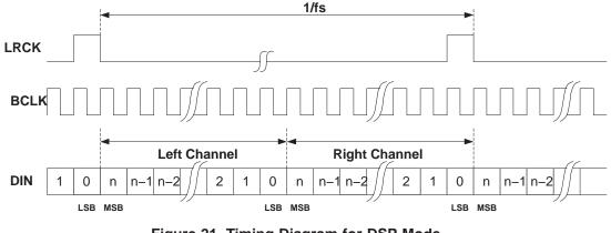
Figure 21. Timing Diagram for DSP Mode
