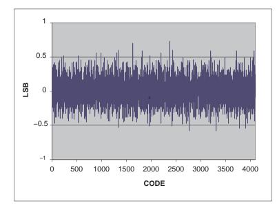
Figure 6. SAR DNL (T<sub>A</sub> = 25°C, Internal Ref = 2.5 V, AVDD = 3.3 V)
