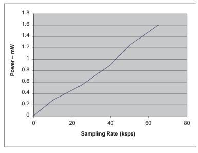
Figure 7. Touch Screen Power Consumption With Speed ( $T_A = 25^{\circ}C$ , External Ref, Host Controlled AUX Conversion, AVDD = 3.3 V)
