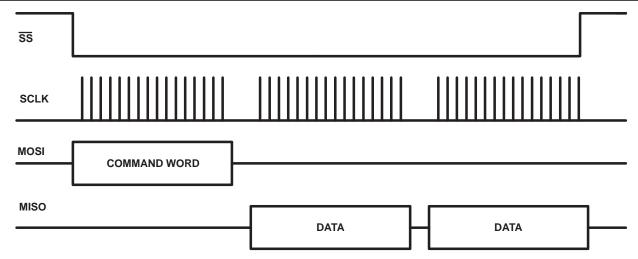
Figure 25. Read Operation for TSC2102 SPI Interface
