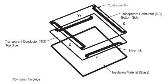
Figure 10. 4-Wire Touch Screen Construction
