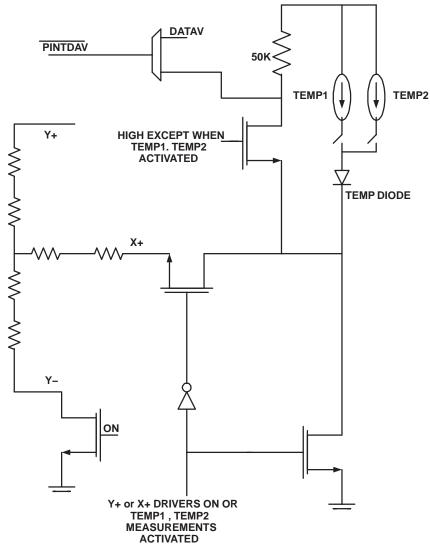
Figure 13. PINTDAV Functional Block Diagram
