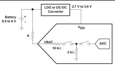
Figure 17. Battery Measurement Functional Block Diagram
