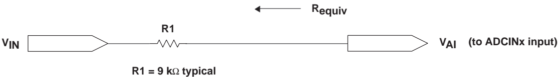
Figure 47. Typical ADC Input Pin Circuit
