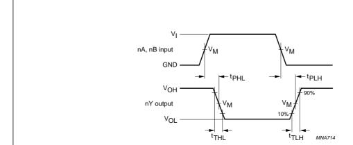
For 74HC2G00:  $V_M$  = 50%;  $V_I$  = GND to  $V_{CC}$ . For 74HCT2G00:  $V_M$  = 1.3 V;  $V_I$  = GND to 3.0 V.
