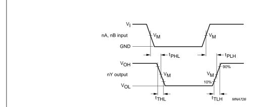
For 74HC2G08:  $V_M$  = 50%;  $V_I$  = GND to  $V_{CC}$ . For 74HCT2G08:  $V_M$  = 1.3 V;  $V_I$  = GND to 3.0 V.
