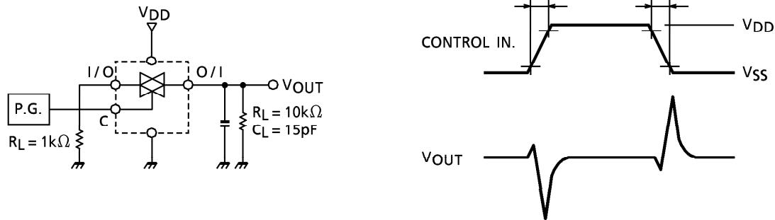
7. TOTAL HARMONIC DISTORTION, f<sub>MAX</sub> (I / O-O / I), FEEDTHROUGH (SWITCH OFF)
